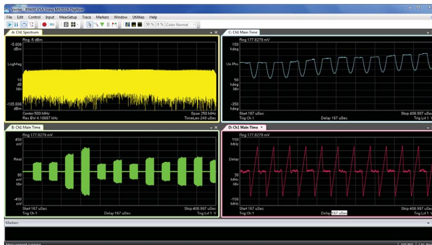
Figure 13. Spectrum, phase, frequency, and time domain displays of a chirped radar signal using the Agilent 89600 VSA software and the M9392A PXI Vector Signal Analyzer.
